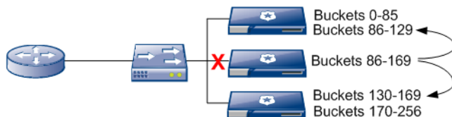
Figure 1-8 Automatic Redistribution of Loads
