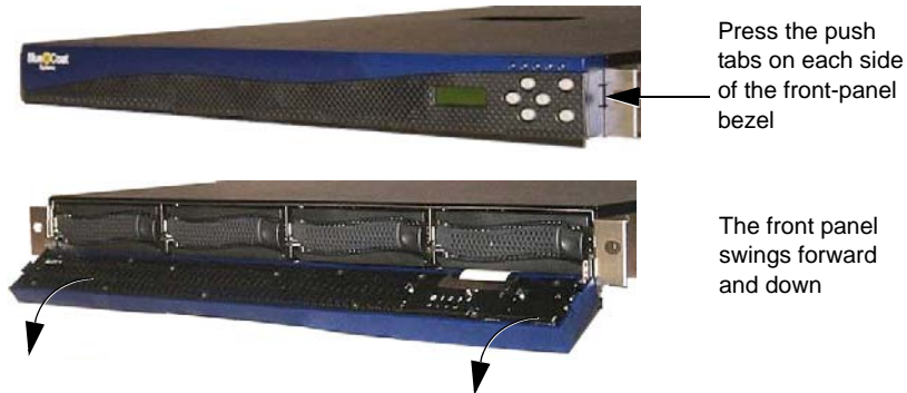
Figure 1-6: Access the Disk Drive Slots
