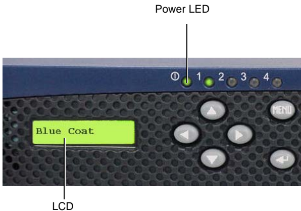
Figure 5-1: SG810 Powering Up
